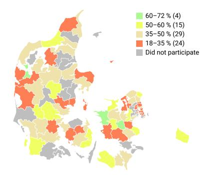
Figure 2 The above map shows the distribution of municipal roads according to lifespan in 2017. Municipalities colored in grey did not participate in the assessment. Green indicates municipalities with a low maintenance debt, while red indicates municipalities with a high maintenance debt.
